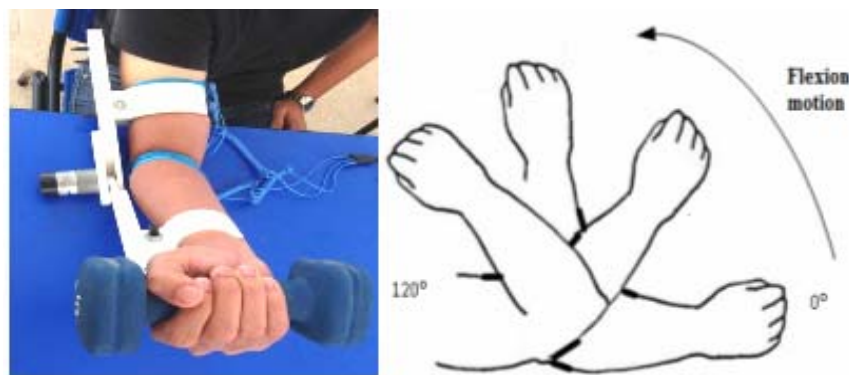
Figure-2. Subject is set-up with arm rehabilitation assistive device for experiment (a). Simulation of subject's to lift up the dumbbell 5 pounds of weight (b).
