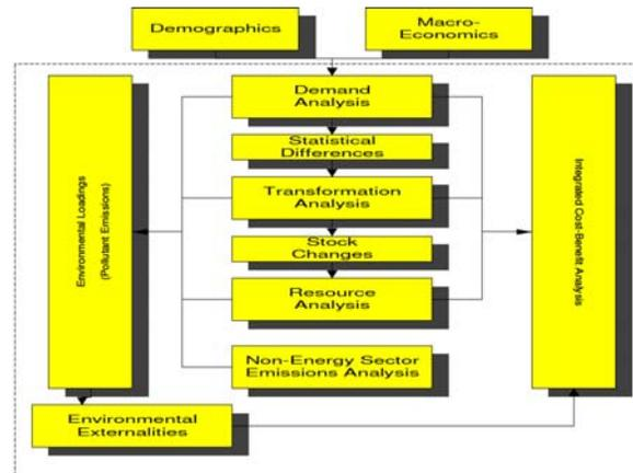
Figure-4. LEAP Structure and calculation flows [13].
