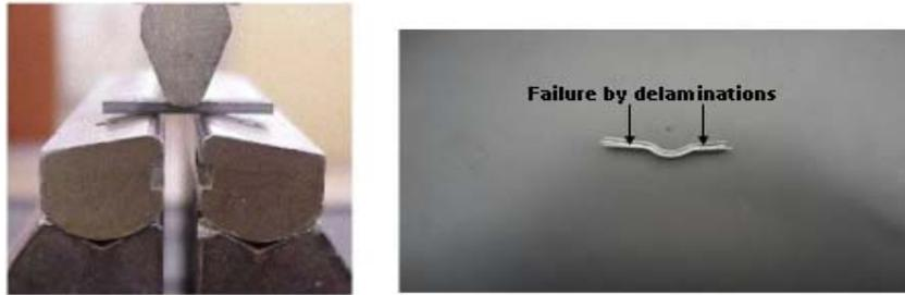
**Figure-7.** Shear test arrangement and tested specimen.
