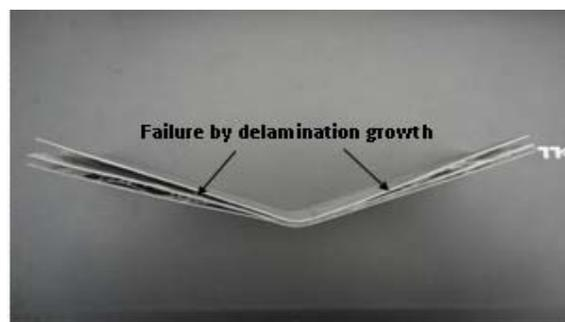
**Figure-8.** Inter-laminar fracture tested specimen.
