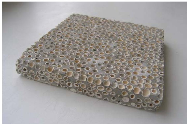
Figure-3. The sample of constructive heat-insulating lightweight concrete with NGA after filing.
