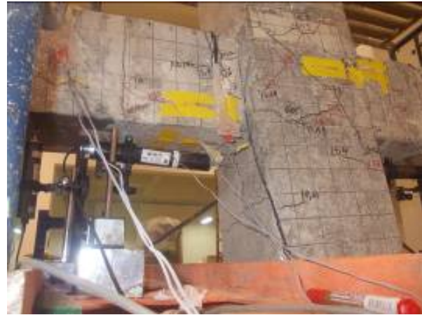
Figure-12. Crack pattern of PC specimen.
