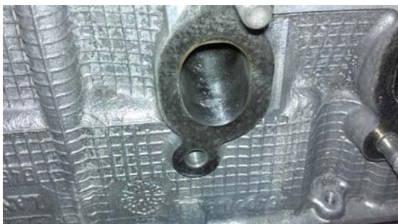
Figure-11. Ribs and stringers in the casting of the head of a FIAT "Fire" engine.
