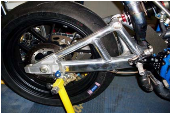
Figure-10. Rosmoto SR 744R's swing-arm, cast, machined and tubular parts are welded together.
