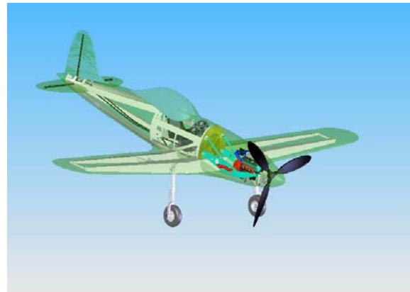
Figure-5. The "black replica" of the Macchi 205 with transparent skin and fins. The single-rubber-bladder MIL-DTL-27422 fuel tank behind the Orenda engine is not shown. It is bolted directly to the front bulkhead.
