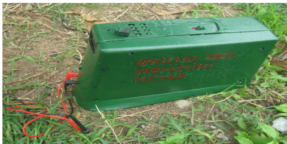
Figure-2. The assembled digital soil moisture meter.
