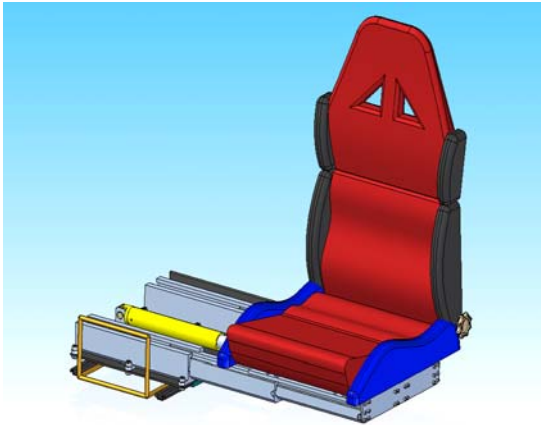
Figure-9. Sturdy, compact and simple design of the seat. Unfortunately this seat cannot rotate.
