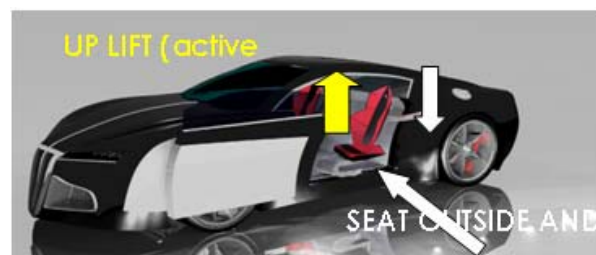
Figure-3. The sliding door: the seat is in the "entrance position", with the bar outside, the seat outside and rotated.
