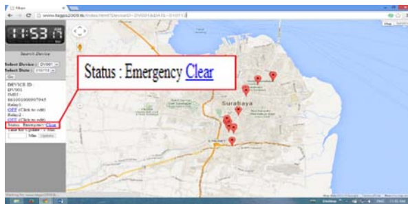
Figure-8. Markers of the location of the vehicle when the vehicle travels for some period of time are shown. Note also the Emergency button status is clear.
