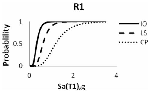
Figure-8. Fragility curves of the structure retrofitted by RC jacking.
