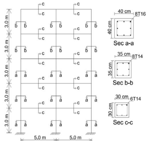
Figure-3. Typical 5-story RC frame and the sections of beams and columns.
