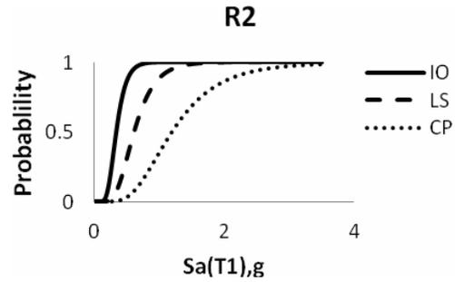
Figure-9. Fragility curves of the structure retrofitted by steel jacking.
