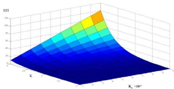
**Figure-12.** 3D plot of EFI of the retrofitted frame (R1) vs. the hazard curve parameters ( $k$  and  $k_0$ ).
