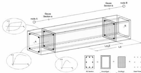
**Figure-4.** Discretization of typical RC cross section in Seismostruct.
