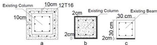
**Figure-5.** Three retrofit methods used in this study
