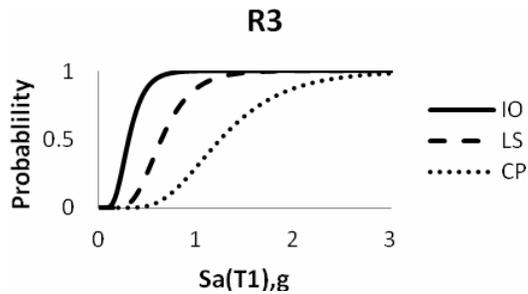
Figure-10. Fragility curve of the structure retrofitted by CFRP Wrapping.
