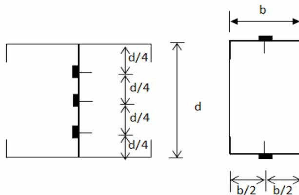
Figure-4. BTB and BU screw position on the column section.
