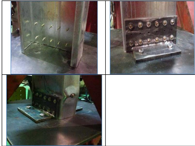
**Figure-5.** Simple support of self-drill screw through the plate to the web at both column ends.
