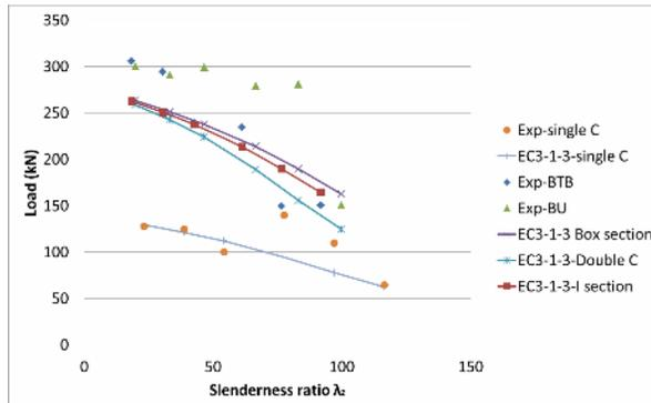
**Figure-6.** Ultimate capacity of cold formed steel (CFS) column.
