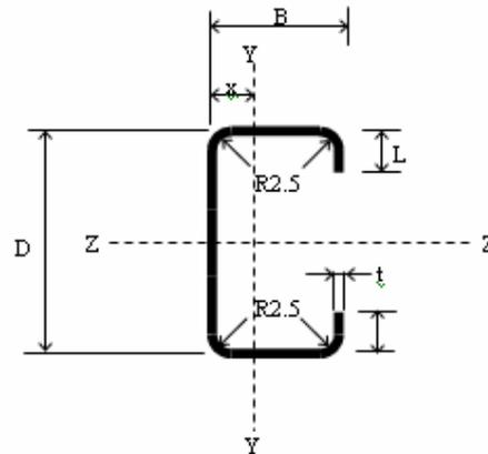
**Figure-2.** Dimension of CFS.
