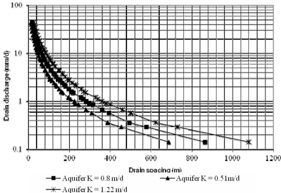
**Figure-4.** Relationship between design drain spacing and drain discharge for different aquifers.
