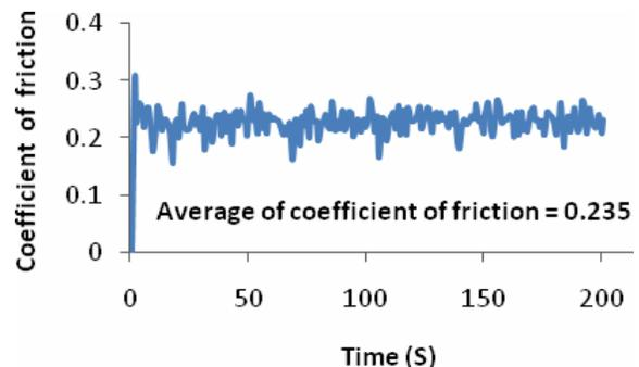
**Figure-2.** An example of coefficient of friction record shows the average of coefficient of friction with sliding speed 15 m/s and contact pressure 1 MPa (for specimen of composite 30% PR).
