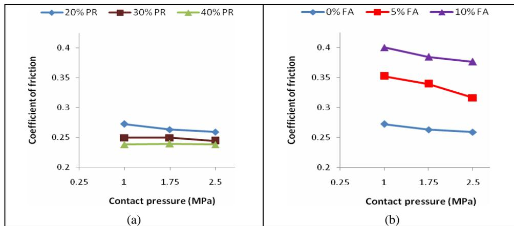
**Figure-3.** Effect of: (a) phenolic resin, and (b) fly ash on coefficient of friction toward variation of contact pressure (with sliding speed 5 m/s).
