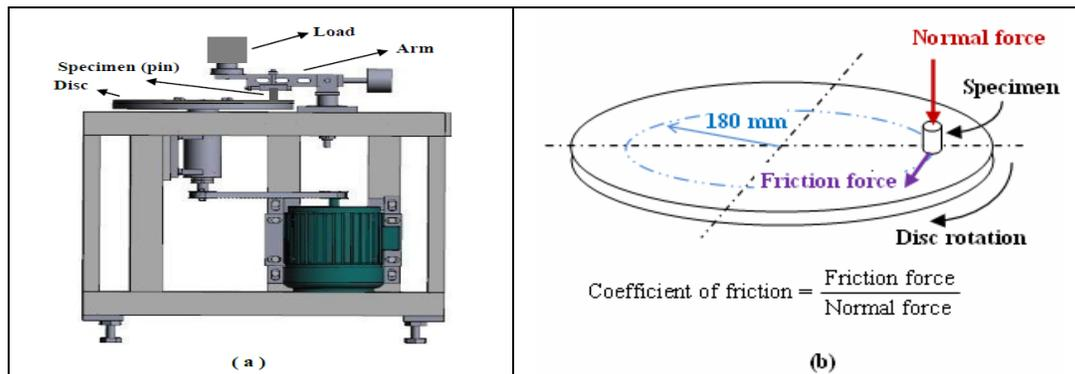
**Figure-1.** Test set up of friction wear testing: (a) schematic of pin on disc machine, (b) the friction force acts on contact surface.
