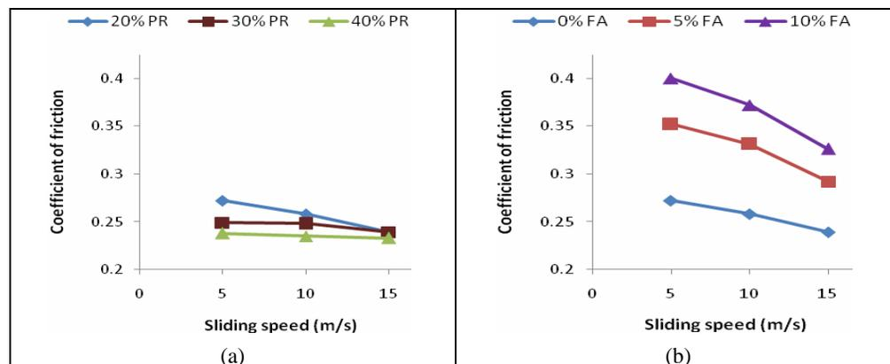
**Figure-4.** Effect of: (a) phenolic resin, and (b) fly ash on coefficient of friction toward variation of sliding speed (with contact pressure 1 MPa).
