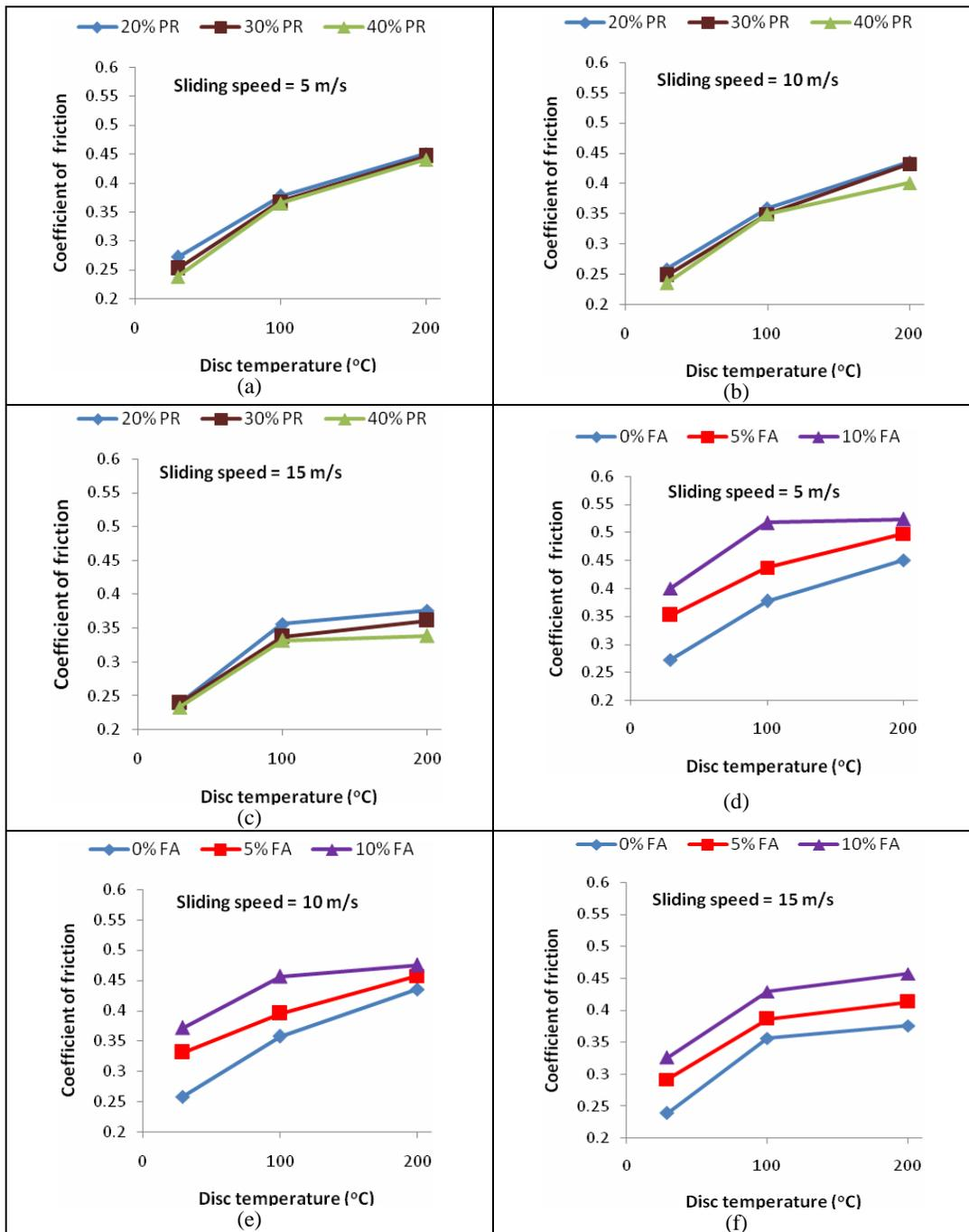
**Figure-5.** Effect of phenolic resin (a, b, and c) and fly ash (d, e, and f) for 1 MPa of contact pressure on coefficient of friction toward variation of disc temperature and sliding speed.
