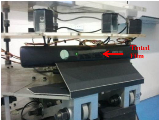
Figure-14. Tinted film at Kinect sensor.
