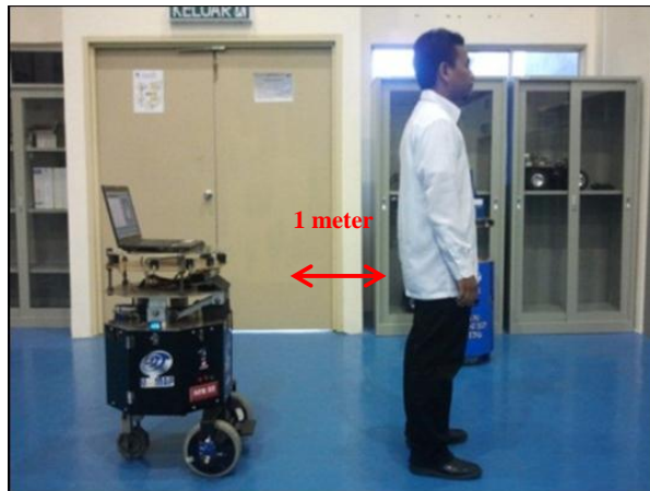
Figure-11. Distance for robot to stop.
