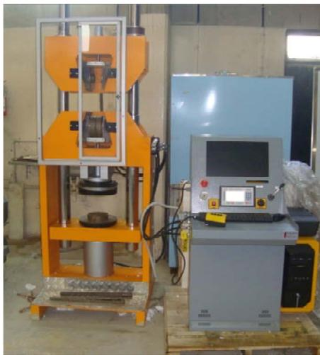
Figure-5. Universal tensile and compression tester model: UBCH-001.
