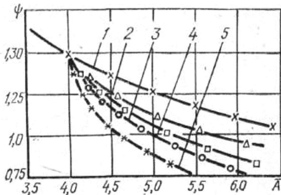
**Figure-3.** Impact of the lubricant kind on the friction factor behavior during operation: 1- initial curve (statics); 2 - fluid lubricant; 3 - solid lubricant; 4 - consistent lubricant; 5 - lubricant in the supply state.
