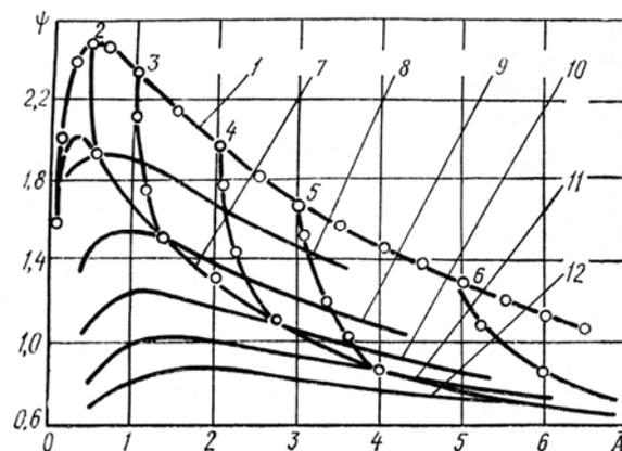
**Figure-1.** Dependence of the coefficient of the energy dissipation in the material on the relative strain amplitude during operation.
