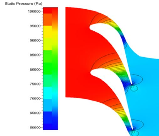
Figure-3. Field of static pressure at the mid-section of the nozzle diaphragm.
