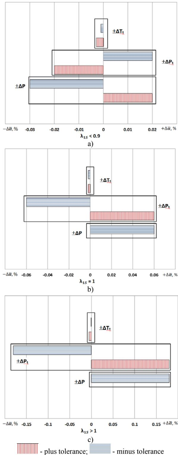
**Figure-14.** Impact of change of physical parameters of the blade row under consideration on the reduced angle of the flow exit from the grid at  $\lambda_{1s} < 0,9$  (a),  $\lambda_{1s} = 1$  (b),  $\lambda_{1s} > 1$  (c).
