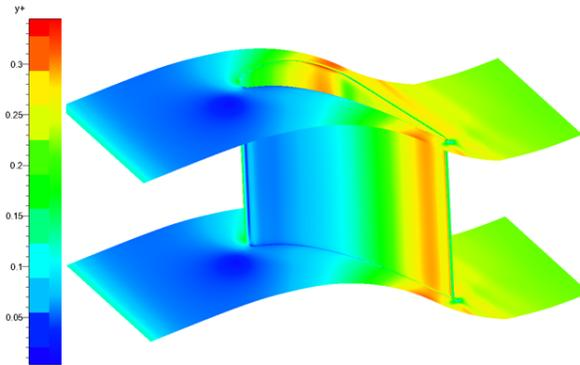
**Figure-5.** Distribution of the  $y^+$  parameter over the blade (c).
