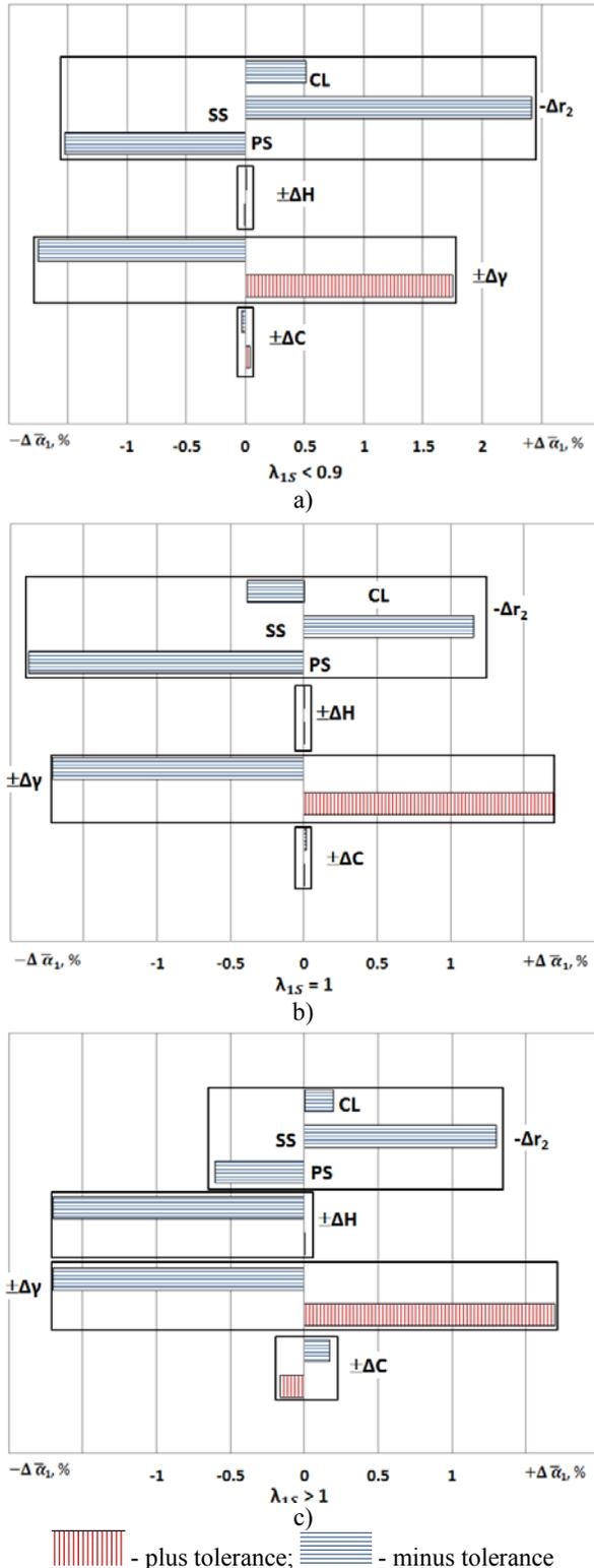
**Figure-10.** Impact of change of geometrical parameters of the blade row under consideration on the specific flow angle at  $\lambda_{1s} < 0,9$  (a),  $\lambda_{1s} = 1$  (b),  $\lambda_{1s} > 1$  (c).
