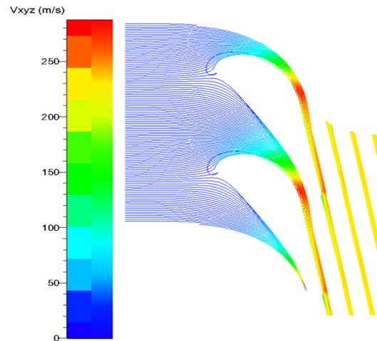
Figure-4. Streamlines at the mid-section of the nozzle diaphragm.
