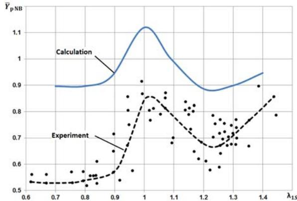
**Figure-6.** Dependence of the specific profile losses on the isentropic flow rate at the cascade outlet.
