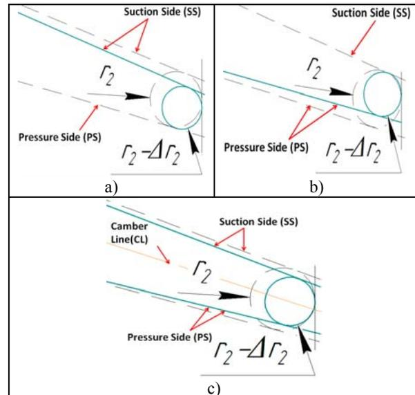
**Figure-7.** The variation of the trailing edge position aligned against the pressure side (a), suction side (b) and camber line (c) of the reference profil by the tolerance value.
