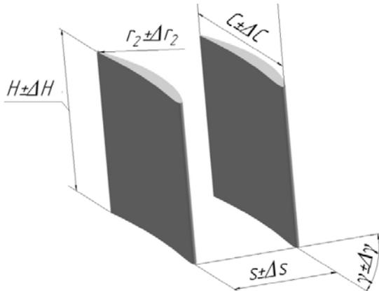
**Figure-1.** Design of the blade row with the most relevant dimensions.
