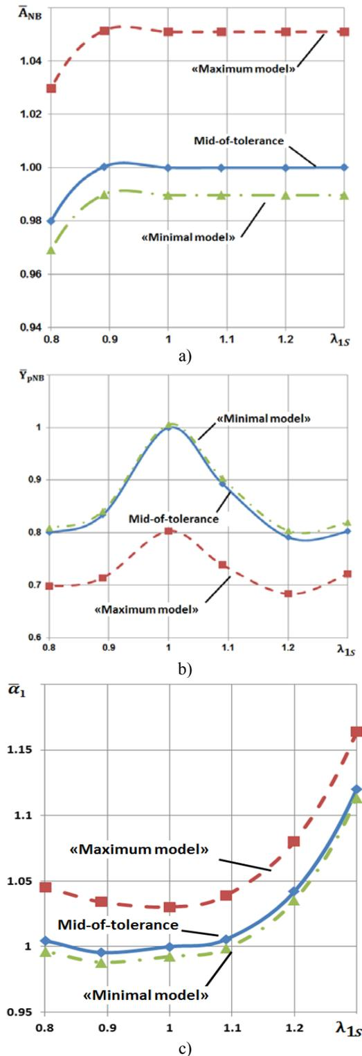
**Figure-11.** Dependence of the specific mass flow parameter (a), specific profile losses (b) and specific angle of the flow exit (c) on the isentropic flow rate at the cascade outlet for the “maximum”, “minimum” and “nominal model”.
