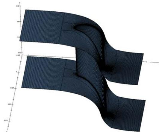
**Figure-2.** The computational domain with the finite-element grid applied.
