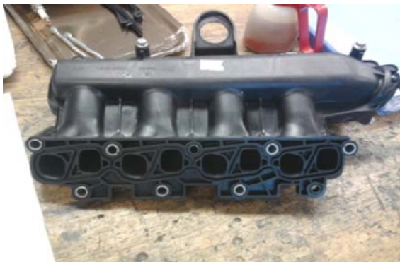
Figure-3. Original intake.
