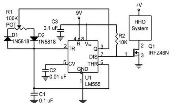
**Figure-3.** Circuit diagram.
