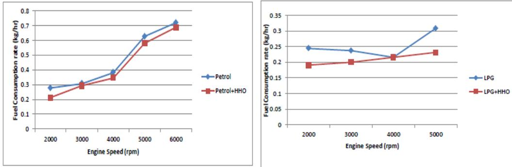
Figure-6. Effect of HHO gas on fuel consumption.
