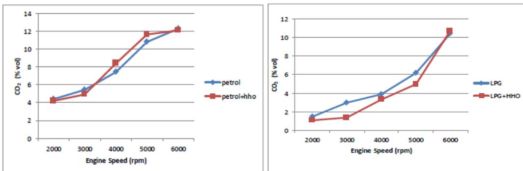
Figure-9. Change in carbon dioxide concentration with engine speed.
