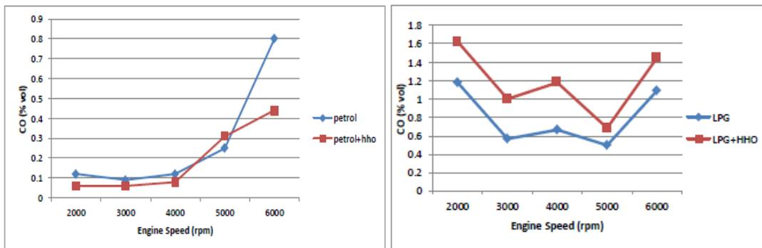
Figure-7. Change in carbon monoxide concentration with engine speed.
