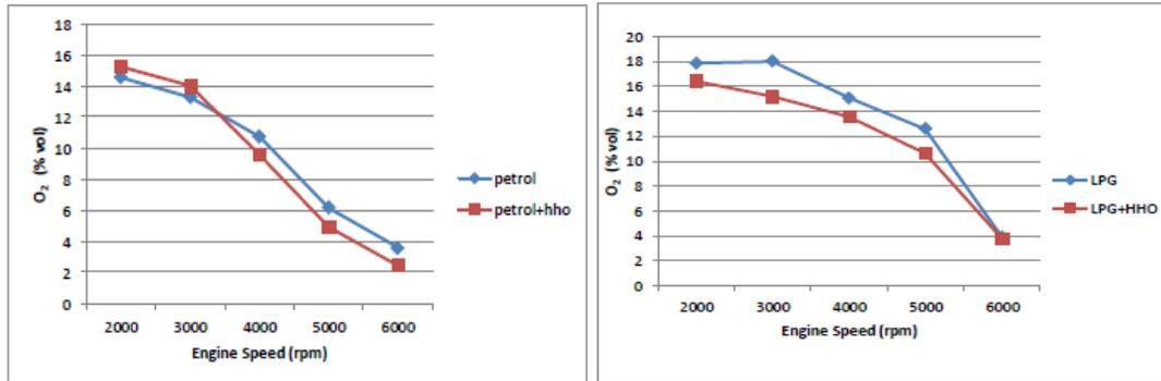
Figure-10. Change in oxygen concentration with engine speed.
