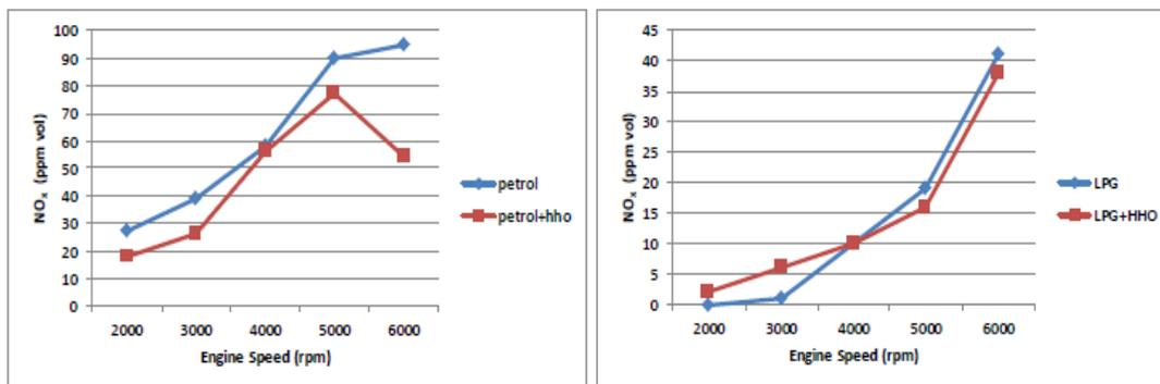
Figure-11. Change in nitrogen oxide concentration with engine speed.
