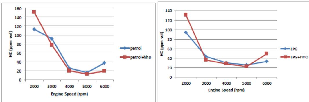
Figure-8. Change in hydro carbon concentration with engine speed.
