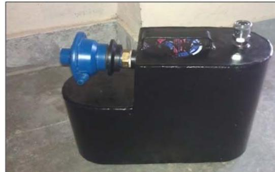
**Figure-2.** LPG storage tank with regulator (blue).
