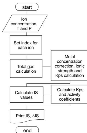
**Figure-2.** Flow chart based on Odco and Tomson model for scale formation prediction.
