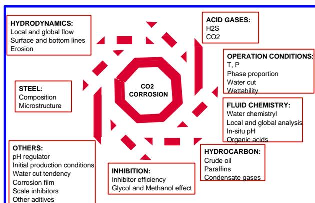
**Figure-1.** Factors affecting CO<sub>2</sub> corrosion. After Kermani and Morshed (2003).
