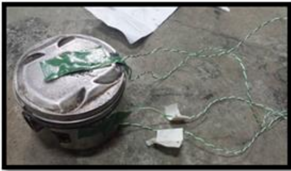
Figure-3. Thermocouple attached to the piston surface using steel epoxy.
