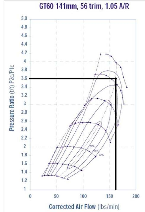
Figure-4. Garrett GT60 Compressor Map (low pressure stage).
