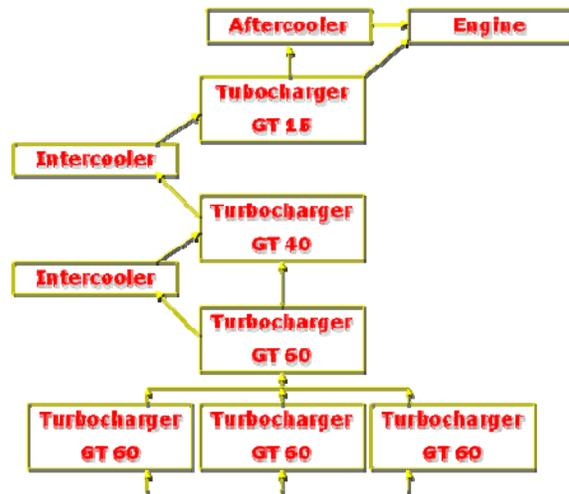
Figure-7. Turbocharging system from 17500m to 2000m.
