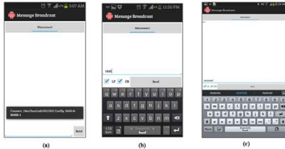
Figure-11. ZigBeeComm broadcast message window: (a) Connection is established with the USB endpoints. (b) Message is broadcasted and (c) received by other devices.
