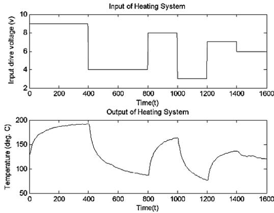
Figure-4. Input and output behavior of heating system.
