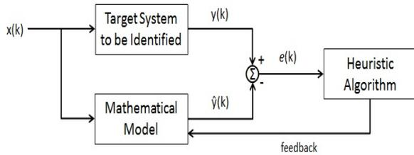
Figure-1. A schematic of system identification problem utilizing the heuristic search algorithms.
