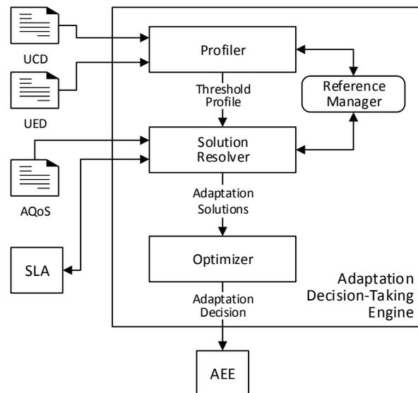
Figure-2. The ADTE architecture based on MPEG-21 DIA.
