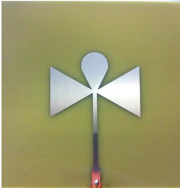
Figure-1.1. The geometry of the Ice Cream Cone with Bow Tie antenna.
