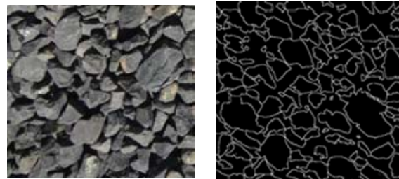
Figure-7. Image of ballast and Watershed transform boundaries.
