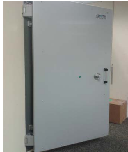
Figure-8. Shield room that is used to measure the performance of CEE in less congested environment.
