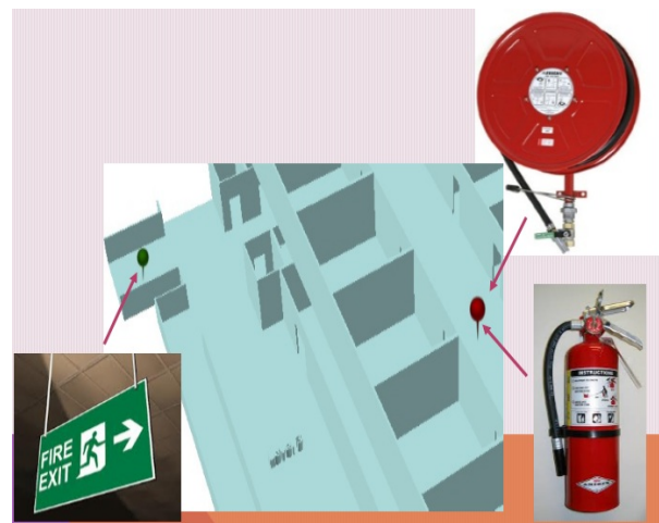
Figure-7. Nearest exit from the sensor and fire hose location.
