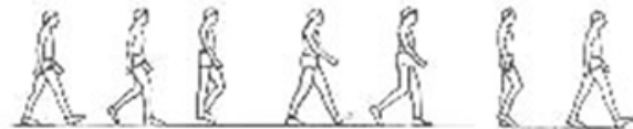
Figure-3. A complete gait cycle that starts from a heel strike and ends at a heel strike of the same leg (Murray, 1967).
