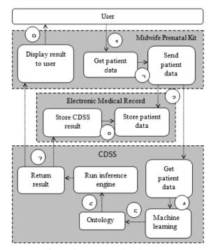
Figure-6. CDSS workflow in IPMS.
