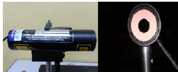
Figure-2(a). Transmitter (Laser Diode) and receiver (receiver lens),
