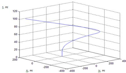
**Figure-8.** Ascent path of the quadrotor under wind effect. Bending of the flight path reflects the influence of wind disturbances on the quad rotor.
