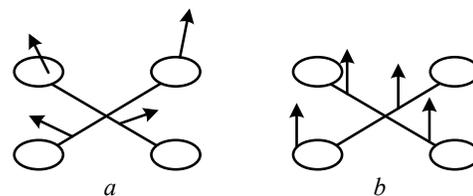
**Figure-1.** Approaches to analysis of wind effect on quad rotor.
