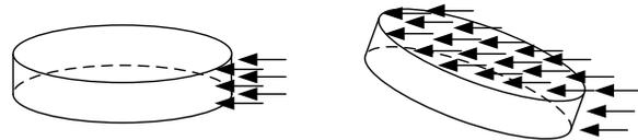
**Figure-7.** Wind effect on a quad rotor construction.
