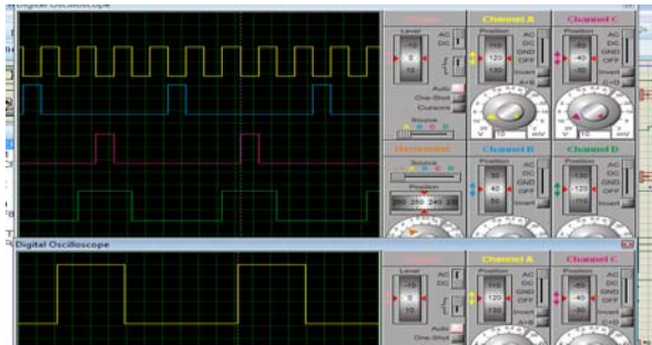
Figure-20. 2 Five level inverter output pulse.
