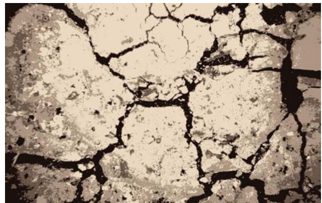
Figure-3. Received image from thin section photo of sample No 58 (Figure-2): pores are black.
