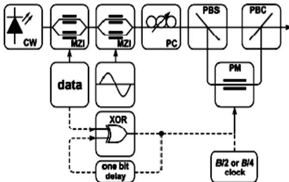
Figure-3. Transmitter schematic of APol CSRZ.
