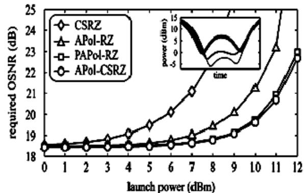
Figure-4. Required OSNR for a BER of 10 versus launch power after transmission over 4\_80 km SSF.
