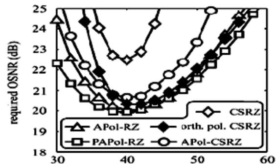
Figure-5. Back-to-back required OSNR versus demultiplexer filter bandwidth for optimized multiplexer filter bandwidth, 3WDM system, 50Hz.
