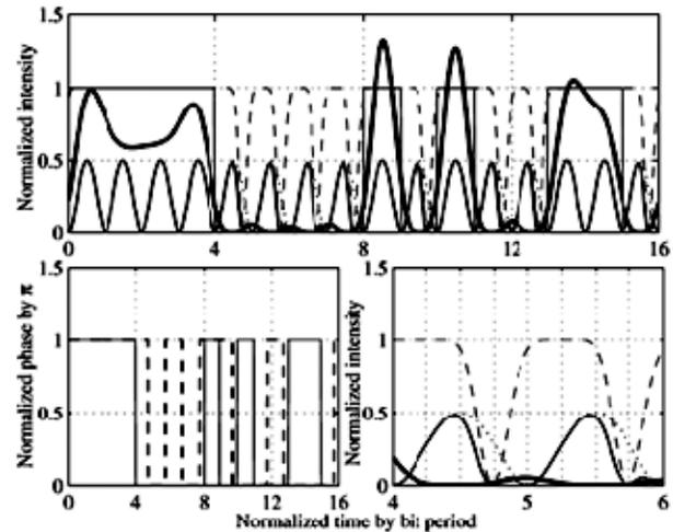
**Figure-7.** Time waveforms of (top) intensity of SSB-DPSK-ACS-RZ signal (solid thick line) and of DPSK-ACS-RZ (solid line) with optimized relative time delay between DPSK (dashed line) and the clock signal (dotted line); (bottom—left-hand side) normalized phase by  $\pi$  of DPSK signal (dashed line); (bottom—right-hand side) enlarged "00" detail of the top plot. The solid thin line represents the *deBruijn* binary sequence
