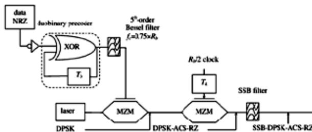
**Figure-6.** Generation scheme of novel SSB-DPSK-ACS-RZ signaling format.
