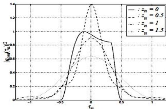
Figure-2. CWSW pulse evolution in a linear lossless fiber.
