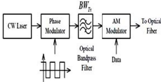
Figure-1. Transmitter block diagram of CWSW.
