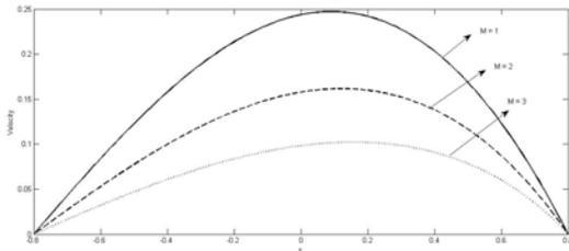
**Figure-4.** Effect of Hartmann number  $M$  on velocity  $u$  with  $a = 0.2$ ,  $b = 1.2$ ,  $d = 2$ ,  $\omega = 1$ ,  $t = 1$ ,  $x = 0.5$ ,  $Re = 1$ ,  $\phi = 0$ ,  $\lambda = 0.001$ ,  $s = 1$ ,  $N = 1$ ,  $Pe = 1$ ,  $Sc = 1$ ,  $K = 1$ ,  $Gc = 1$ ,  $Gr = 1$ ,  $\alpha = 1$ .
