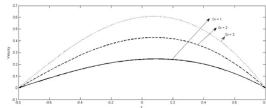
**Figure-1.** Effect of Grashof number for heat transfer  $Gr$  on velocity  $u$  with  $a = 0.2, b = 1.2, d = 2, \omega = 1, t = 1, x = 0.5, Re = 1, \phi = 0, \lambda = 0.001, N = 1, s = 1, M = 1, Pe = 1, Sc = 1, K = 1, G_c = 1, \alpha = 1$ .
