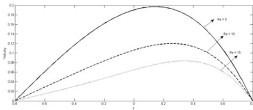
**Figure-5.** Effect of Reynolds number  $Re$  on velocity  $u$  with  $a = 0.2$ ,  $b = 1.2$ ,  $d = 2$ ,  $\omega = 1$ ,  $t = 1$ ,  $x = 0.5$ ,  $\phi = 0$ ,  $\lambda = 0.001$ ,  $s = 1$ ,  $H = 1$ ,  $N = 1$ ,  $Pe = 1$ ,  $Sc = 1$ ,  $K = 1$ ,  $Gc = 1$ ,  $Gr = 1$ ,  $\alpha = 1$ .
