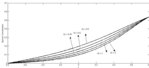
**Figure-6.** Effect of Schmidt number  $Sc$  on Concentration with  $a = 0.2$ ,  $b = 1.2$ ,  $d = 2$ ,  $\omega = 1$ ,  $t = 1$ ,  $x = 0.5$ ,  $\phi = 0$ ,  $\lambda = 0.001$ ,  $s = 1$ ,  $M = 1$ ,  $N = 1$ ,  $Pe = 1$ ,  $Re = 1$ ,  $K = 1$ ,  $Gc = 1$ ,  $Gr = 1$ ,  $\alpha = 1$ .
