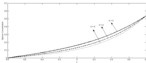
**Figure-7.** Effect of Chemical reaction parameter  $K$  on Concentration with  $a = 0.2$ ,  $b = 1.2$ ,  $d = 2$ ,  $\omega = 1$ ,  $t = 1$ ,  $x = 0.5$ ,  $Re = 1$ ,  $\phi = 0$ ,  $\lambda = 0.001$ ,  $N = 1$ ,  $s = 1$ ,  $H = 1$ ,  $Pe = 1$ ,  $K = 1$ ,  $Gc = 1$ ,  $Gr = 1$ ,  $\alpha = 1$ .
