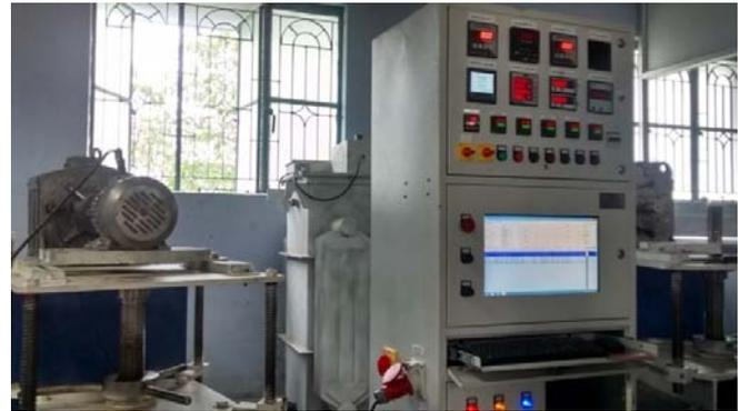
**Figure-9.** Variable load test of SCRIM.
