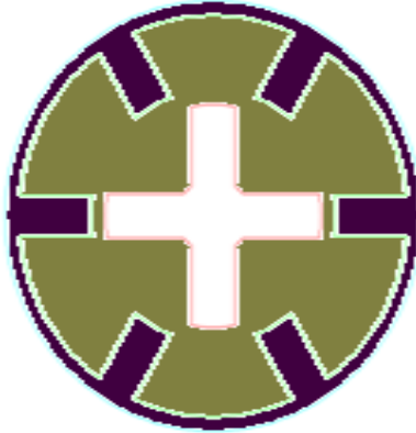
Figure-1. SRM model for 6/4.
