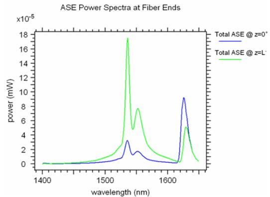
**Figure-7.** Simulated model of ASE Noise in EDFA at Fiber ends of the optical communication system.
