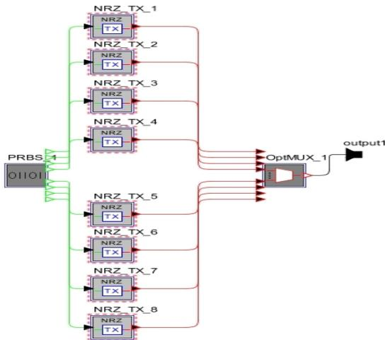
**Figure-4.** Single NRZ 16 channels Transmitter (look inside in simulation model as NRZ\_TX16).
