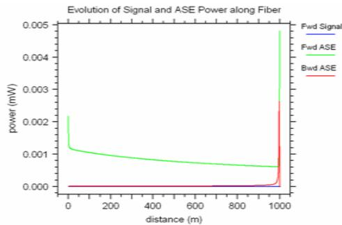
**Figure-5.** Simulated model of EDFA ASE Noise Development using single Pumping scheme.
