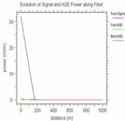
Figure-10. Forward Signal and ASE Noise Characteristics in EYCDFA.
