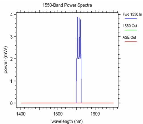
**Figure-9.** Output amplified signal spectrum characteristics of Cascaded simulation model with single pumping.
