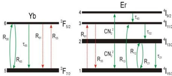
Figure-1. Erbium and ytterbium atomic manifolds.
