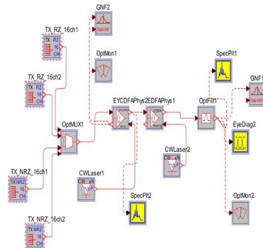
**Figure-3.** Simulation model of proposed work: EDFA cascaded with EYCDFA of single stage (forward) pumping.
