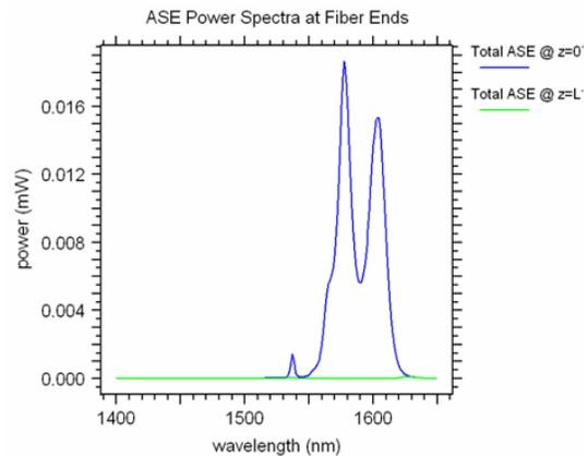
**Figure-8.** Simulated model of EYCDFA ASE Noise at Fiber ends of the optical communication system.
