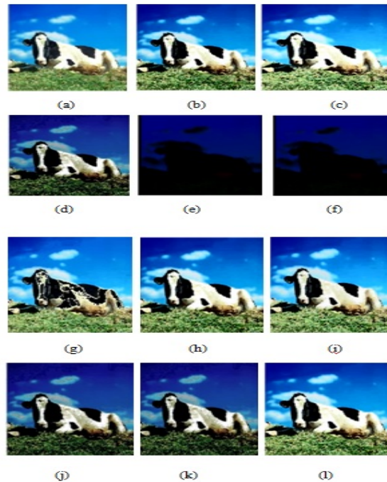
Figure-5. Histogram Equalization output for Cow image (a) Original Image (b) BPBHE (c) DSIHE (d) MMBEBHE (e) AHE (f) CLAHE (g) MHE (h) MPHE (i) WTHe (j) DHE (k) GPHE (l) RMSHE.
