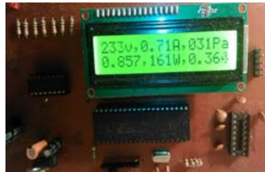
Figure-9. Meter readings under Inductive and resistive load.
