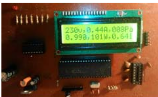
Figure-8. Meter readings under resistive load condition.
