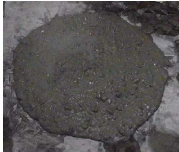
Figure-5. Slump flow the fresh state of SCC uses sea water.
