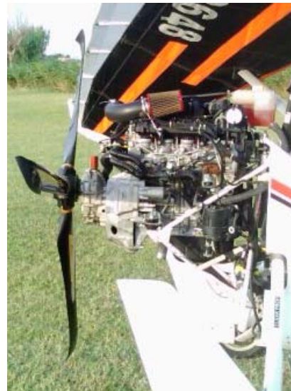
Figure-5. Naldini's trike with CRDID and double rubber joint (2009).
