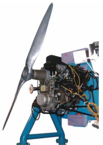
Figure-4. An early installation of the CRF 1900jtd-8V on a propeller-test-bench (2001).
