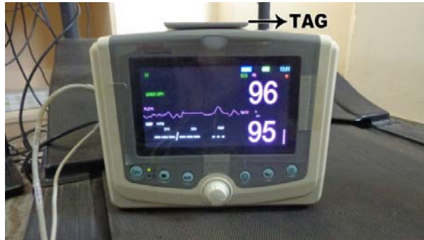
Figure-5. Distortion in pulse oximeter display.
