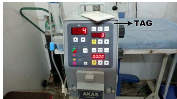
Figure-4. Infusion Pump was tagged with RFID tag.
