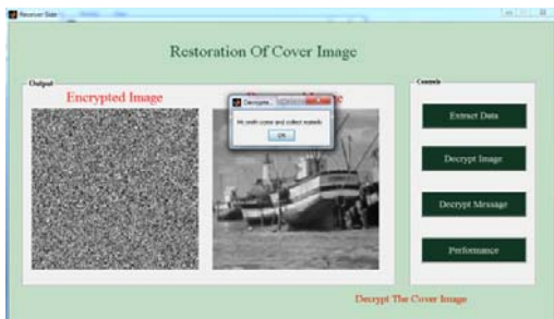
Figure-15. Original secret data and cover image is obtained by decryption and PSNR is 97.6343.
