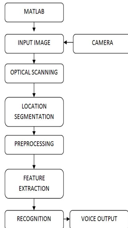
Figure-1. Block Diagram of the text detection using OCR.
