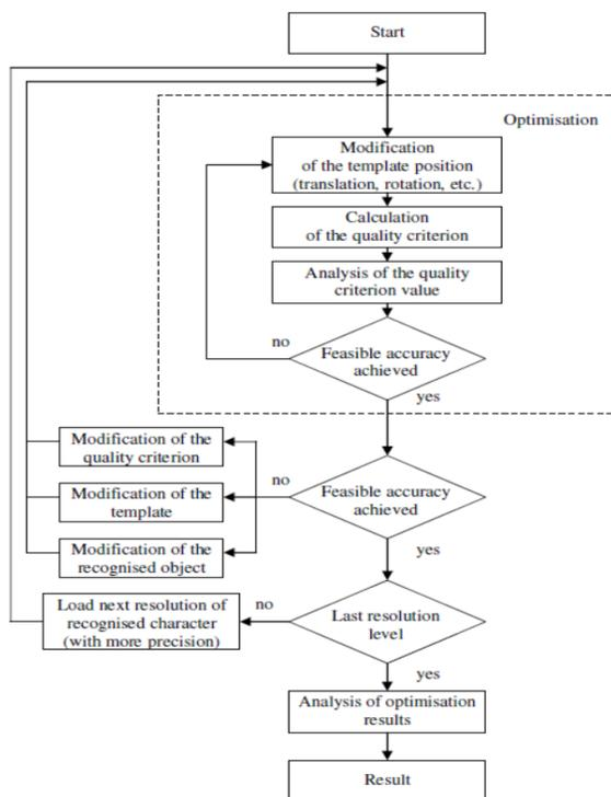
Figure-3. Flowchart for calculation of quality criterion.
