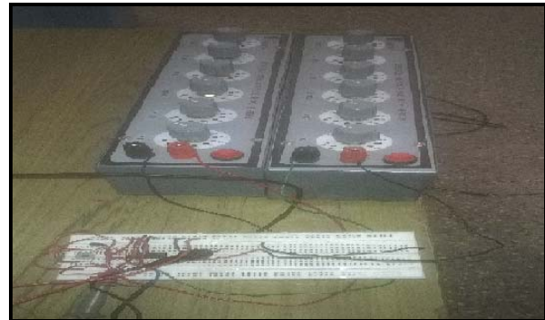
Figure-5. VLC receiver circuit hardware prototype.
