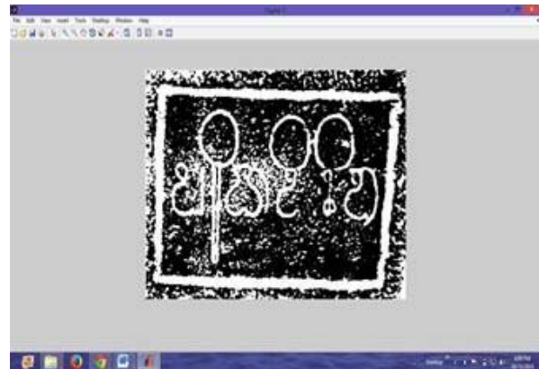
Figure-7. Otsu Thresholding employed after Sobel Edge Detector.
