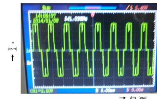
Figure-22. Line to line voltage.
